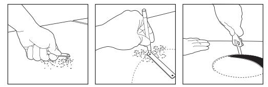
Figure 3. Preparing the Ceiling Tile
